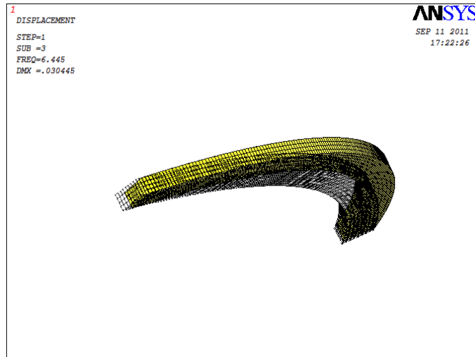
Figure 4.3 Mode shape number 1 of curved beam with [30_2/60_2] laminate
